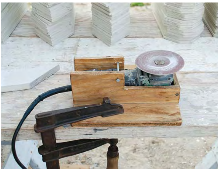
Figure 9. Single edges are eased with a small angle grinder equipped with an 80-grit disc. The tool is enclosed in a plywood box; a large nail holds down the paddle switch.
