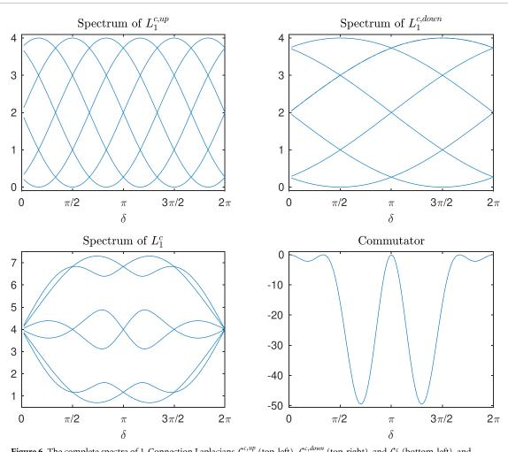
**Figure 6.** The complete spectra of 1-Connection Laplacians  $\mathcal{L}_{1}^{c,up}$  (top-left),  $\mathcal{L}_{1}^{c,down}$  (top-right), and  $\mathcal{L}_{1}^{c}$  (bottom-left), and commutator  $[\mathcal{L}_{1}^{c,up},\mathcal{L}_{1}^{c,down}]$  (bottom-right) for Case 3 directed simplicial triangles is plotted as a function of  $\delta$ .
