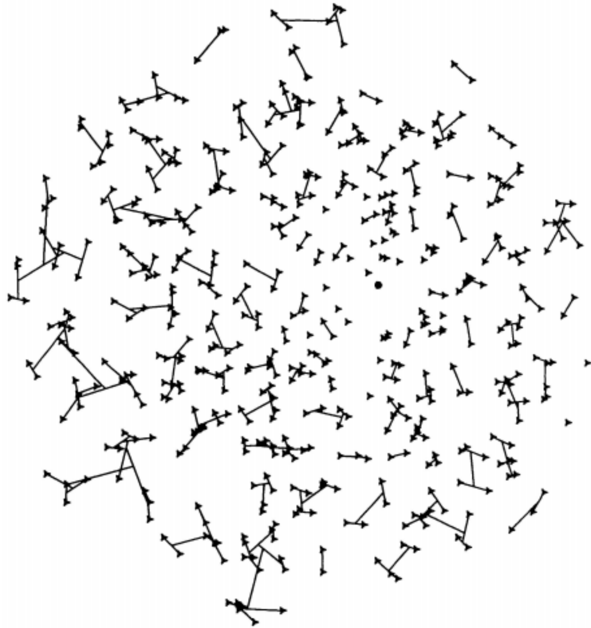
FIG. 6.—Sub-trees corresponding to the force terms generated for the circled particle in a force scan with \Delta A_B = 0.01 . The system consists of 512 particles uniformly distributed in a two-dimensional disk.
