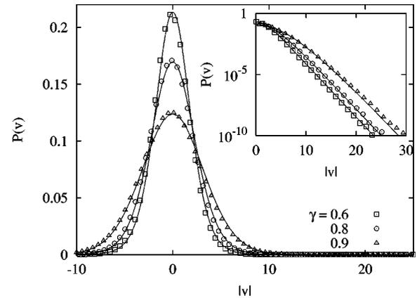
FIG. 2. Velocity distribution  $P(v)$  calculated using Monte Carlo simulations. Simulations were made for  $N=10^5$  particles. Continuous lines are the results obtained from Fourier inversion. The inset shows our data in the semilogarithmic scale.
