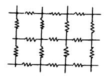
Denote by R(m,n) the resistance between nodes (0,0) and (m,n) in a two-dimensional square lattice of one-ohm resistors. It has long been known that R(m,n) is the integral mean of the doubly periodic function
